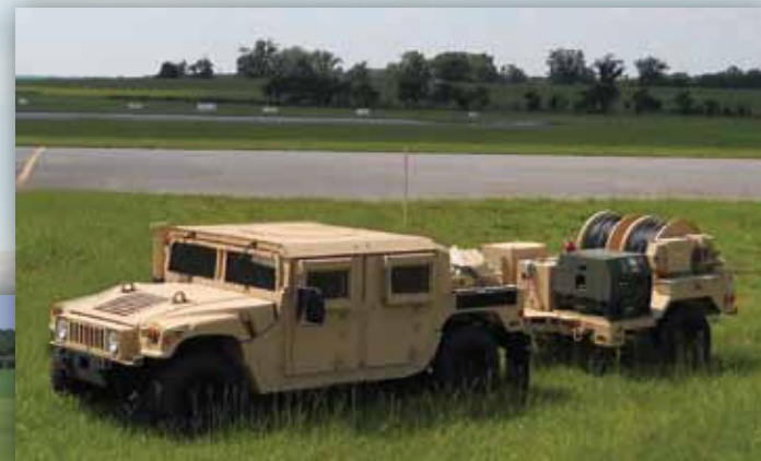
ALS Mover 1: M1165A1 Armored HMMWV Towing Ancillary Airfield Lighting System Equipment and Generator
