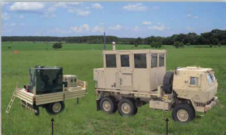
Generator/Equipment Trailer: M1082A1 2.5 Ton LMTV Cargo Trailer Carrying Tactical Quiet Generators & Ancillary Communications Equipment
